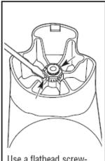
Use a flathead screwdriver to bend up two opposing tabs on the tab washer.
