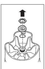
Remove the nut by turning counterclockwise by hand. Then remove the tab washer and pressure washer.
