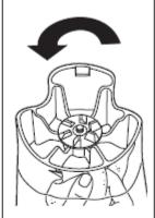
Hold the blades with a cloth. Unscrew the clutch counterclockwise.
