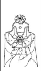
Remove the clutch and felt washer.
