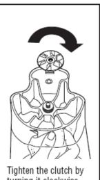
turning it clockwise while holding the blades with a cloth.
