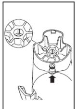
Align the groove in the bushing with the rib on the pitcher and press into place from inside the pitcher.
