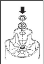
Install the pressure washer, tab washer, and retainer nut by hand. Do NOT overtighten the retainer nut!
